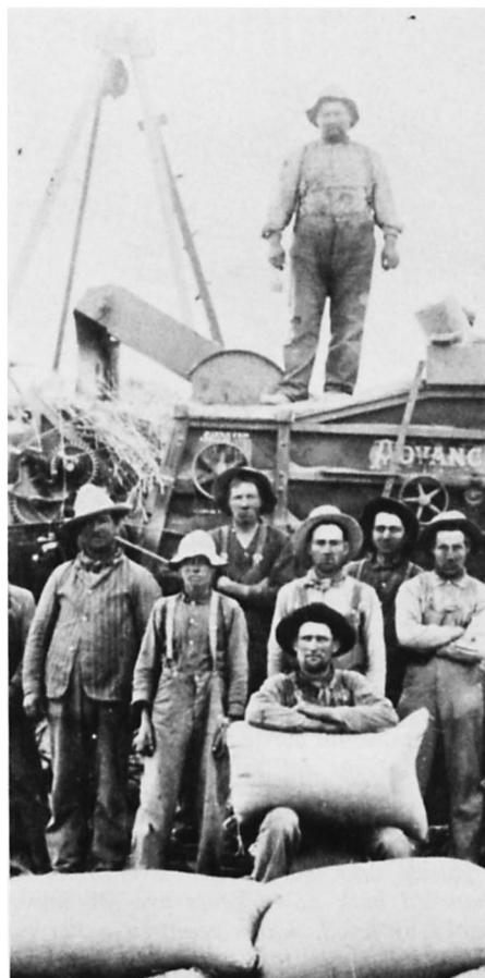
This threshing crew poses in front of its thresher built around 1900 by the Advance Thresher Company of Battle Creek, Michigan. Operated by PTO (power take-off) belt, the separator, by means of a series of shaking screens, separated the grain (in bags, foreground) from the straw.
