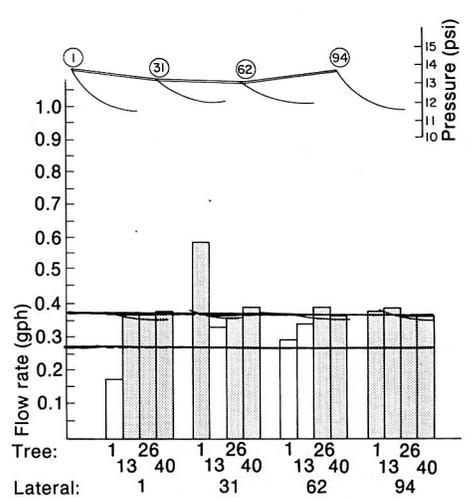
Fig. 5. When emitter plugging is a problem, lowest quarter of discharges tends to be randomly distributed.
