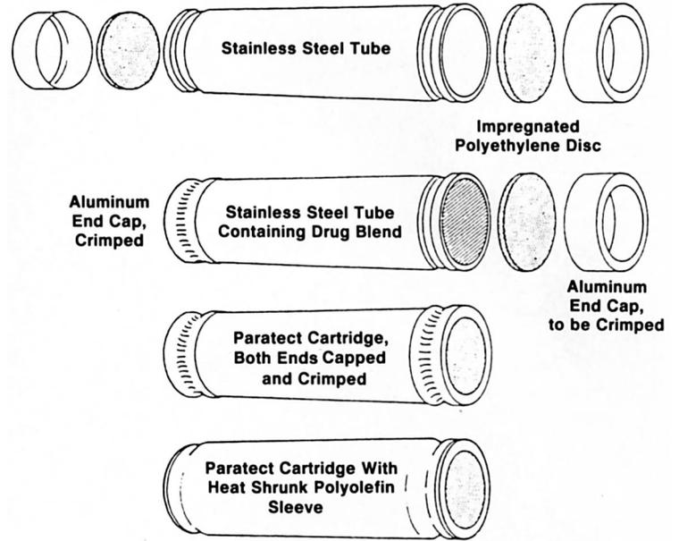
The stainless steel tube contains the deworming medication in an inert polyethylene glycol carrier, which is released through permeable polyethylene diffusion discs at each end. The entire device is enclosed in a heat-shrunk polyolefin sleeve.
