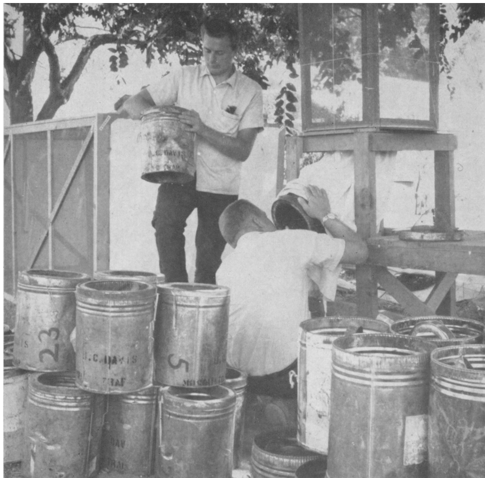
Fig. 4. Blowing mosquito catch from metal trap through cloth sleeve up into holding cage.
