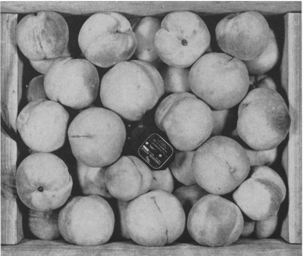
Fig. 8. A vibration pickup positioned in a lug box of peaches.
