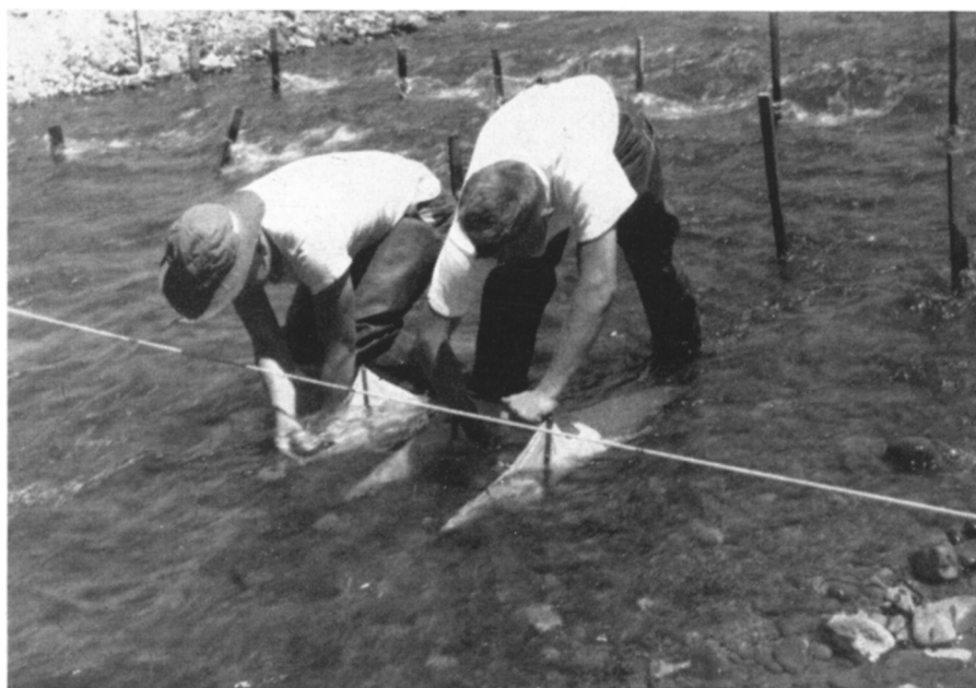
Fig. 2. Sampling technique, using the Surber square foot bottom sampler.
