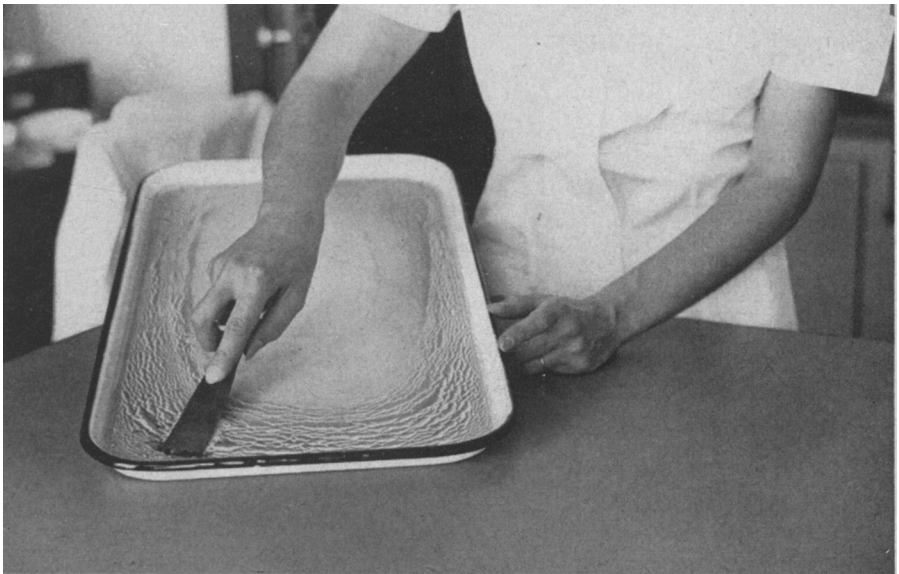
Fig. 7. Spore material after drying in pan and about to be scraped off as powder.
